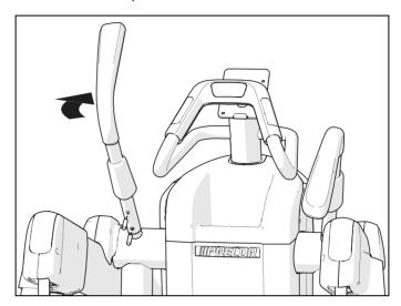
Figure 20: Handlebar positioning steps
