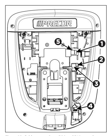
Figure 33: Cable connections, P30 and P10 consoles
