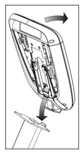
Figure 31: Console positioning on base unit
