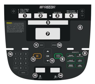
Figure 4: P30 console keys
