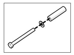
Figure 3: Adding the sleeve and washer
