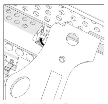
Figure 30: Connecting the power cable
