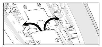
Figure 32: Cable routing from the mount into the console
