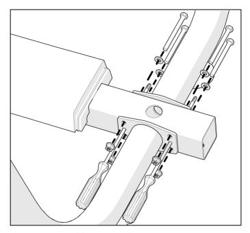
Figure 6: Lower side arm attachment
