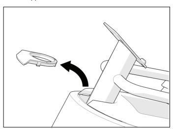
Figure 10: Moisture seal removal
