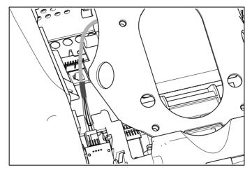
Figure 29: Connecting the heart rate cable
