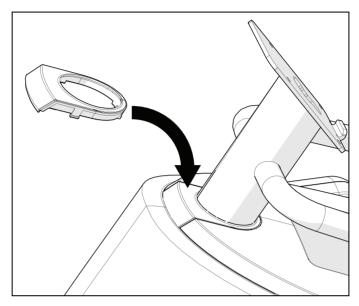
Figure 18: Moisture seal positioning
