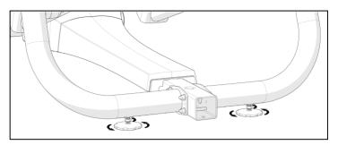
Figure 22: Location of adjustable feet and jam nuts
