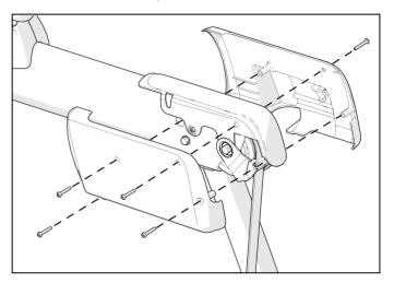
Figure 8: Side arm cover attachment
