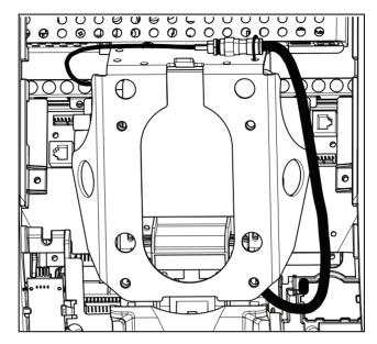
Figure 27: Connecting the television cable
