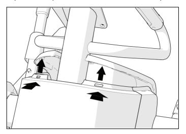
Figure 11: Top cover removal
