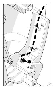
Figure 14: Cable routing through the lower cable channel
