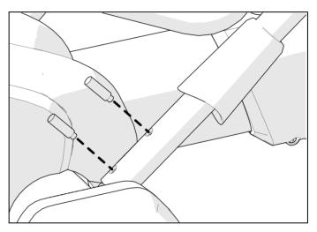
Figure 19: Handlebar set screw removal
