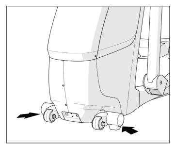
Figure 9: Front pallet anchor locations
