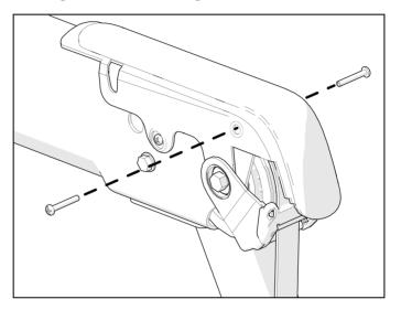
Figure 7: Removal of screws from inner plastic molding
