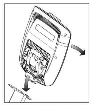
Figure 25: Console positioning on base unit
