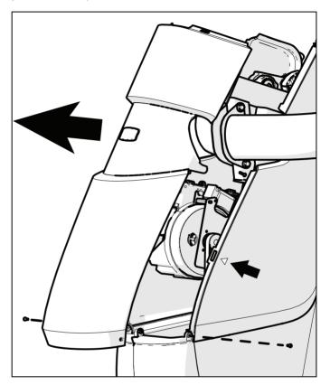
Figure 13: Front cover assembly removal
